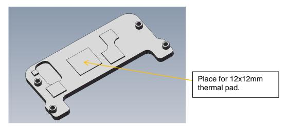
Assemble the heat spreader on top side of the VAR-SOM-OM44. Use the mechanical holes in order to align the heat spreader to VAR-SOM-OM44 PCB.
